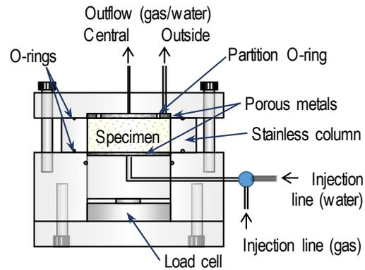
Fig. 3 column test equipment
