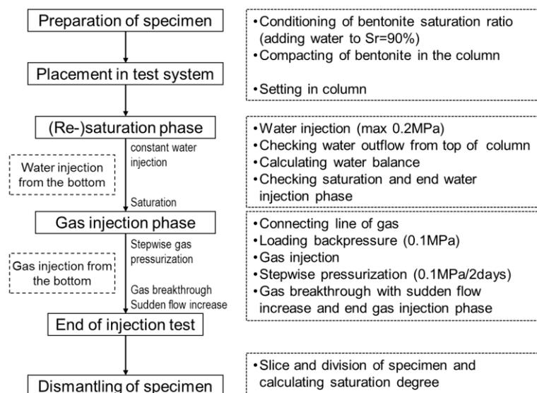
Fig. 5 Flow chart of test procedure
