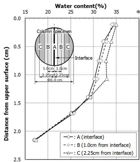
Fig. 10 Measurement of water content inside the bentonite Case-2, after saturation (left), and after breakthrough (right)
